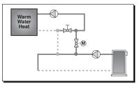
On / Off Injection output is used to operate an on / off device, such as a valve or a pump, in order to inject heat into a constant circulating low temperature loop. This type of mixing requires a differential in order to pre-
