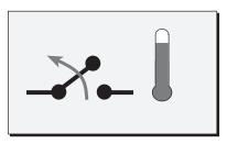
When the slab and outdoor temperatures are warm enough, the snow melting system should automatically turn off. The Warm Weather Cut Off (WWCO) function automatically shuts off the system when snow melt-
