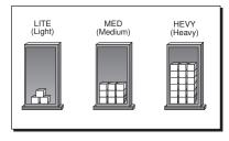
The heat up and cool down rate of a boiler depends on how much thermal mass the boiler contains. By knowing how fast the boiler heats up and cools down, the control can more accurately determine the required
