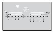
In snow melting systems accurate control of the slab surface temperature is required in order to provide an energy efficient system. When a snow melting slab operates at a higher temperature, the percentage of energy lost
