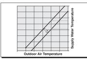
When setback is required, the water temperature to the system should be decreased to provide less heat into the space. tekmar Reset Controls shift the heating curve down in order to provide lower water temperatures
