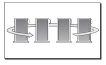
This function rotates the firing sequence of a group of staged boilers based on the accumulated running hours of each stage. When one stage has accumulated 48 hours more running time than any other stage, the oper-
