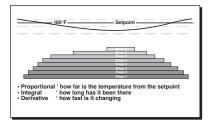
To provide proper boiler staging and accurate boiler supply temperatures, PID (Proportional, Integral, Derivative) control logic should be used. With PID control logic, the number of boilers fired depends on how far the
