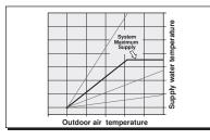
Some systems such as radiant floor heating must be maintained below an allowable maximum temperature in order to protect the tubing or flooring surface. System protection can be achieved by limiting the supply water
