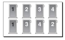
When multiple boilers are staged and rotated the first boiler can be fixed to be fired first at all times. This function allows the boiler nearest to the chimney to create sufficient draft to prime the chimney. This function can
