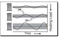
In order to decrease temperature swings and increase boiler efficiency, this function automatically changes the on / off differential of the boiler based on the heating load. As the load increase, the differential will decrease to
